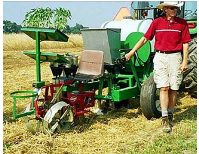
Sub-surface tiller transplanter (photo credit: Mark Schonbeck, Virginia Association for Biological Farming)
