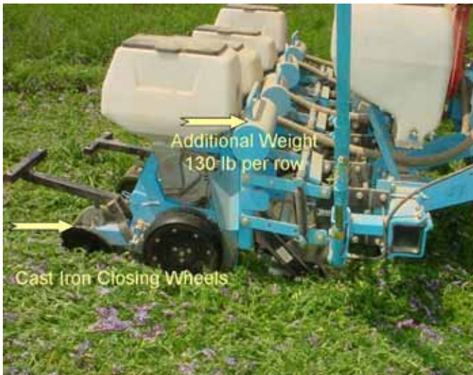
No-till Monosem planter with modifications
