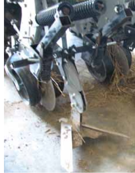
Coulter disc and angled sweep
